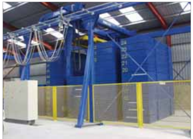
Mould store with portal robot
