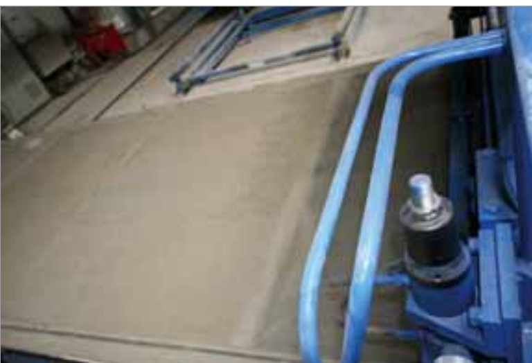
Concrete is highly compacted and flush with the mould
