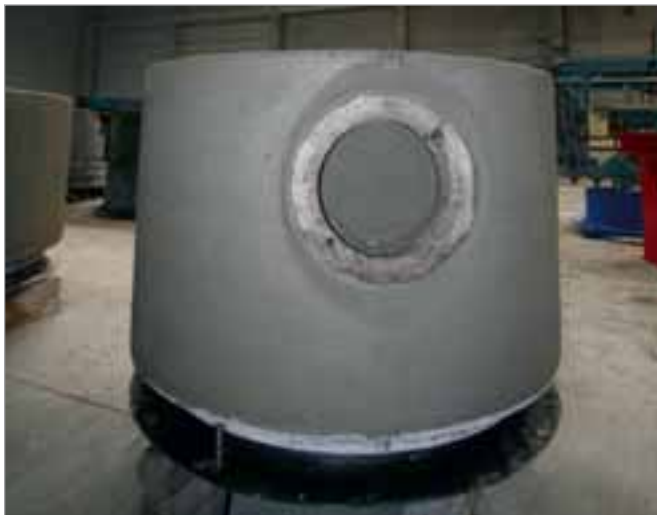
The monolithic manhole bottom rests on steel pallets and support cores in an inverted position during manufacture and further transport.
