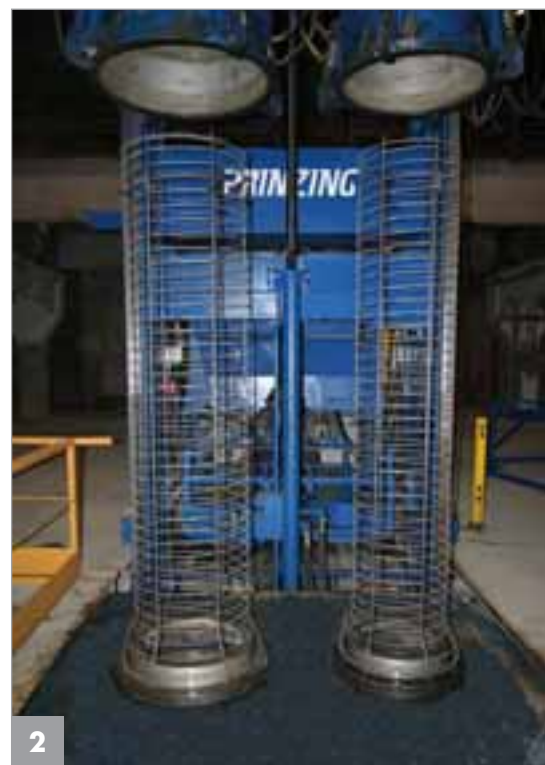
Stable steel cages for the pipes and manhole rings, produced on a new wire-cage machine from MBK
