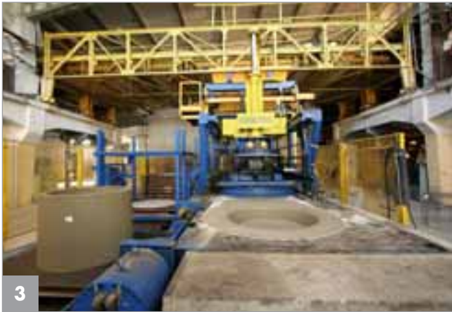
Manufacture of manhole bottoms and tops with just one mould using the tilting table method
