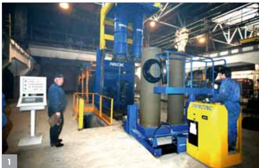
Double production with two different nominal diameters per cycle
