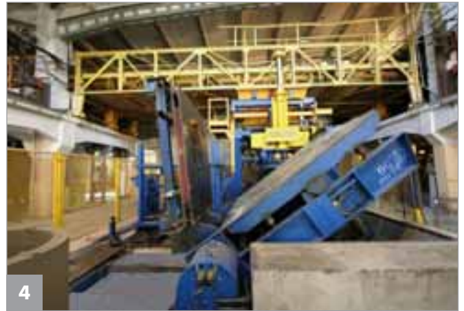
Manufacture of manhole bottoms and tops with just one mould using the tilting table method
