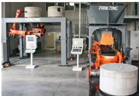
Fig. 1 The new process developed by Prinzing enables the production of monolithic manhole bases.
