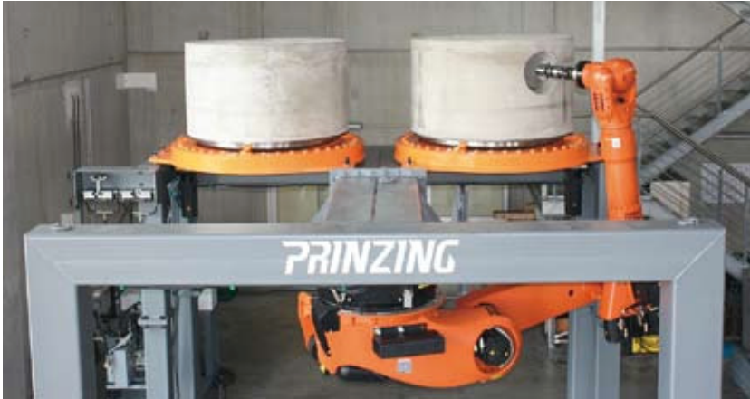
Fig. 7 The pipe connections are also formed with high precision by the milling robot.
