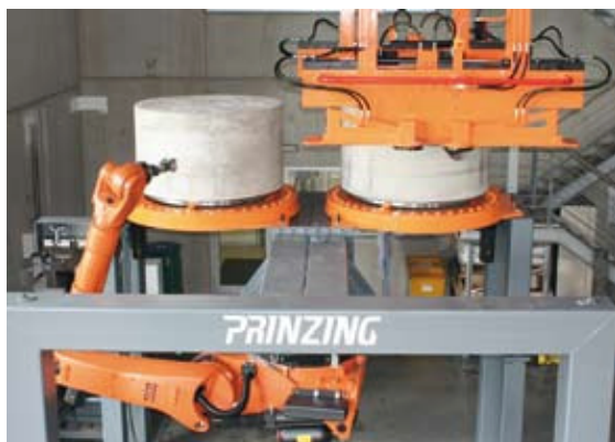
Fig. 5 Manufacturing of the blanks and milling of the drains is completed in brief time intervals.
