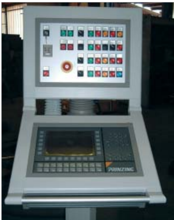
Only one menu-driven control panel which can be rotated in all viewing directions is necessary for the entire manhole pipe plant
