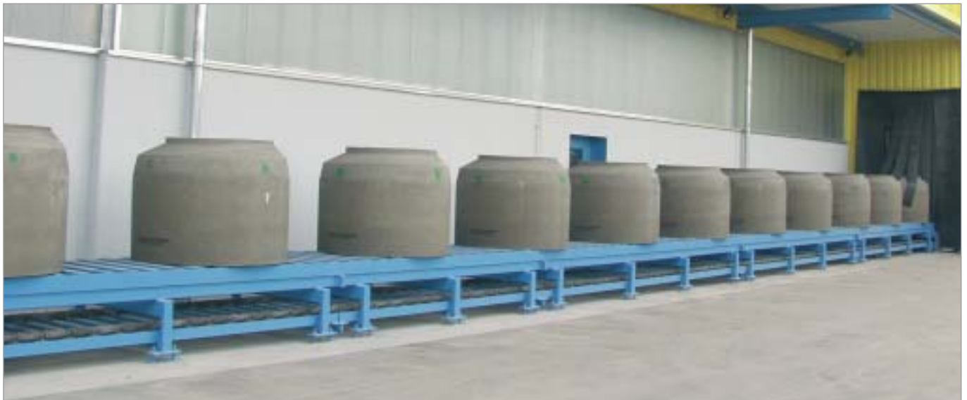
Buffer line for finished products in the outer area of the production hall
