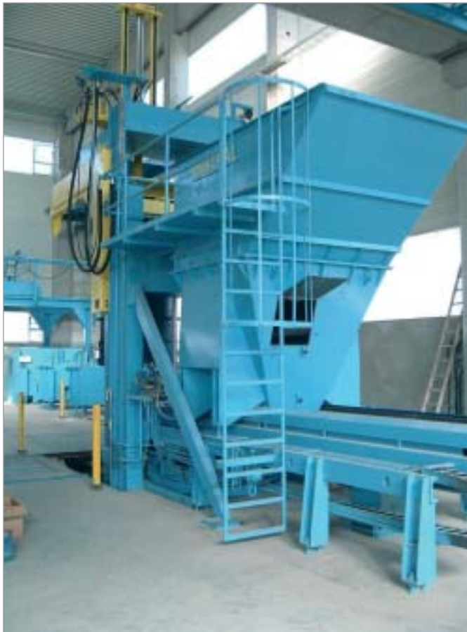
Type MISTRAL 150/250 fully automatic vibration pipe and manhole ring machine
