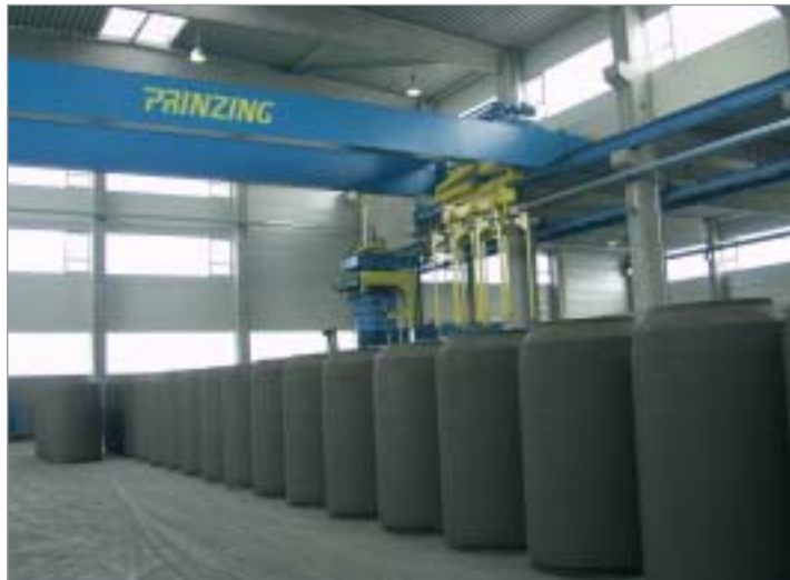
Manhole pipes overall length 2,400 mm with integrated cone and step irons
