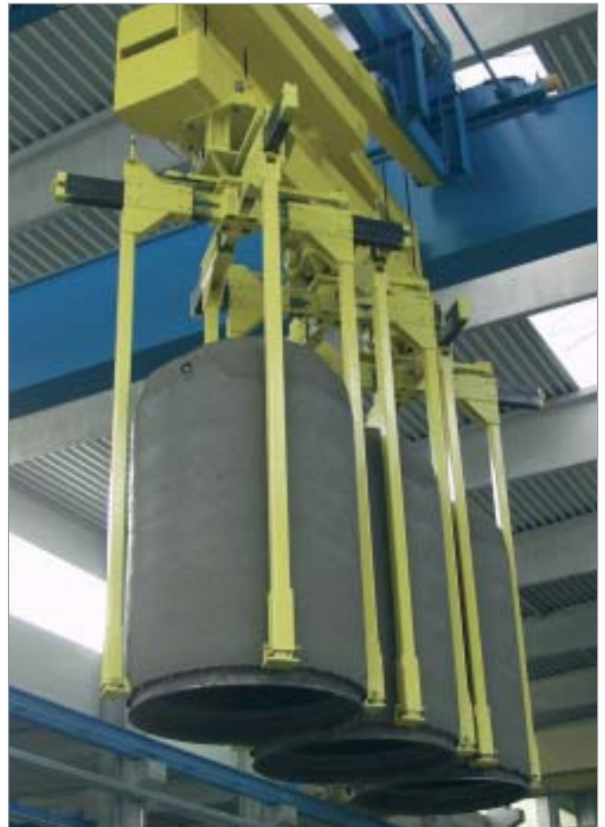
Crane robot with three grippers for the wet and dry end
