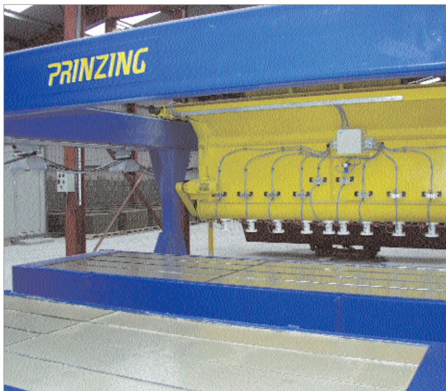
Fully automatic management of up to 130 battery forms in an eight hour shift
