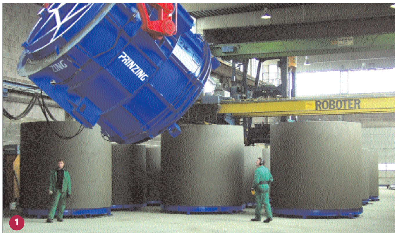
ATLAS laid out for the cost-effective production of concrete tanks
