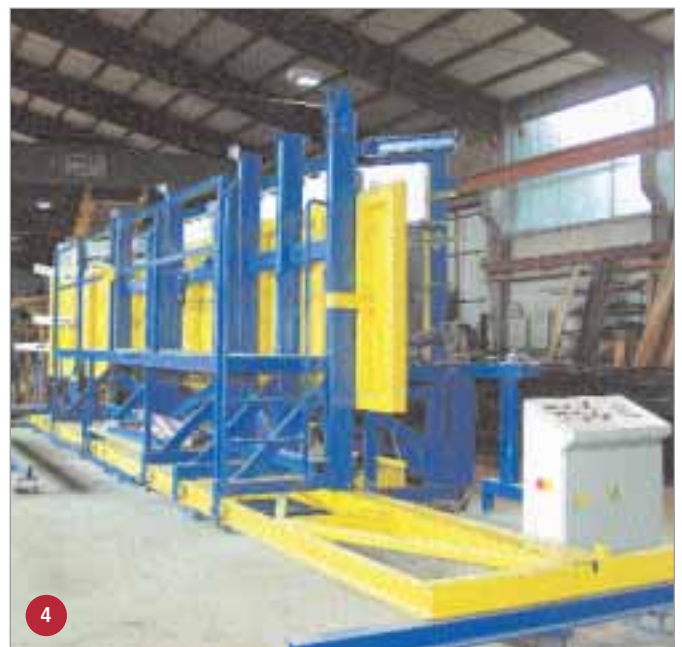
The thickness of the steps and the width of the staircase can quickly be adjusted continuously using guide rails.
