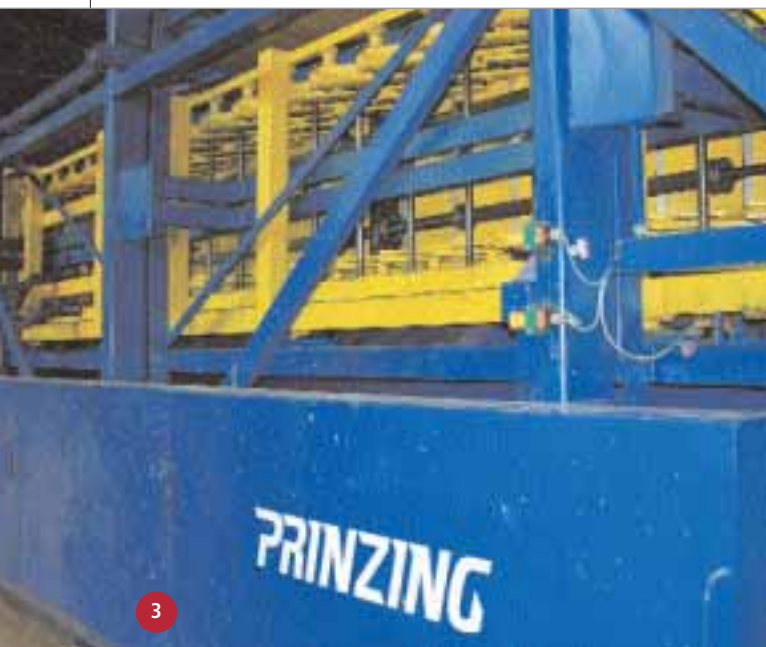
Absolute value sensors mounted on the mold ensure the high degree of dimensional precision of the stairs.
