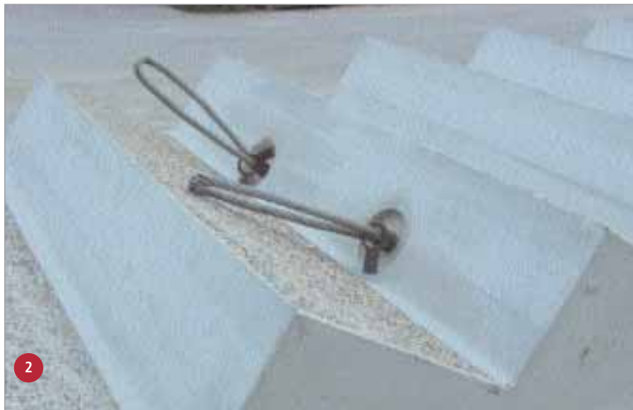
The conversion of the stair mold to another rise angle according to DIN18065 is accomplished in only a few seconds using electric motors.
