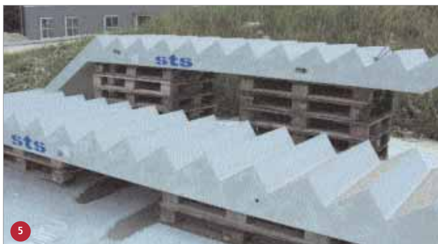
The upper and lower landings can be cast in one process with the stairs.
